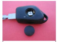
**3.** Remove any remnants of the old rubber key button from outside of remote (no need to open remote) and press fit new Silicone button in.
